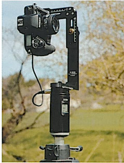
The vertical positioning of the camera makes it possible to capture a significantly higher vertical angle than in horizontal position.
