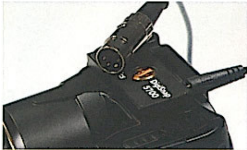
A connection cable between engine and camera allows to control the bracketing and release of the camera.
